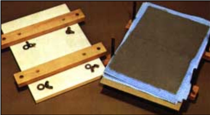
Fig. 10 The completed post is now ready for pressing.
