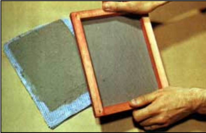
Fig. 9 Couching a second layer of pulp onto the previous one to produce a thicker sheet of paper.
